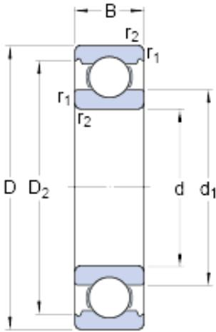
6206 Bearing 2D drawings and 3D CAD models
